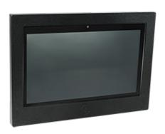
The Touch is a wall-mounted touch screen that gives you switching, dimming and scene control for all your zones. This display measures a full 10" and requires no internet access, communicating with other Lightcloud devices over a wireless mesh network.
